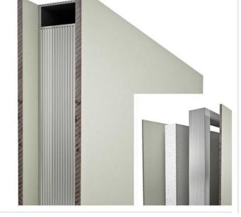
Pharmaceutical grade walls are a covenient and effective solution. They are externally coated on both sides with a melamine laminate sheet, 4 mm thick. Internally, an insulating layer of polystyrene, or a honeycomb structure, between a laminated aluminum frame. Total thickness 45mm.
