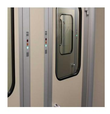
The pharmaceutical door panels are assembled with the same panels as the wall system. The outer frames are made with rounded profiles in anodized or epoxy coated aluminum with double airtight gaskets. All fasteners for hinges and catches can be recessed into the door frame.
