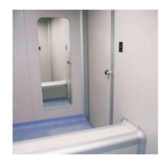
In the changing rooms there are usually ventilated wardrobes for placing clothes and footwear; a bench divides the changing area, so that the operator changes one shoe at a time, bypassing the "grey area" to the clean area. Also, there must be a hand wash or hand sanitizing system, and a mirror, to check proper clothing.
