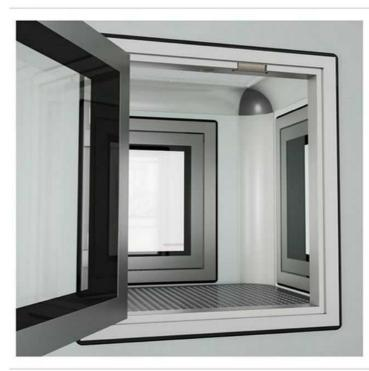
These equipment are specifically designed for the transfer of materials between classified areas or between a classified area and a non-classified area, with decontamination using HEPA filtered air. The ventilation system provides filtered air to ensure a clean environment inside the chamber, before the opening of the door.
