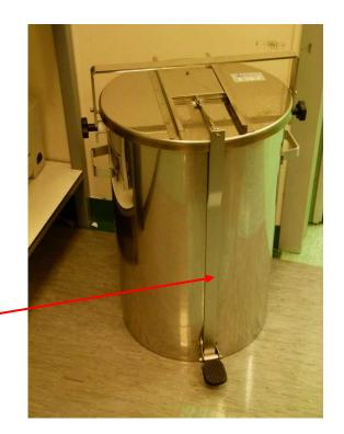
lever control operated by a pedal, which avoids manual opening
