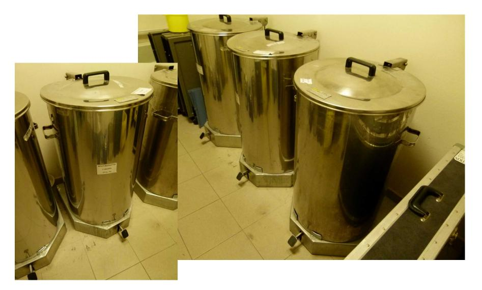
Example: several shielded secondary containers, each containing a suitable primary container, used for the separate collection of waste with increasing half-life. Also note the shielded bags containing the old Co-57 flood sources, awaiting collection by an authorized company.
