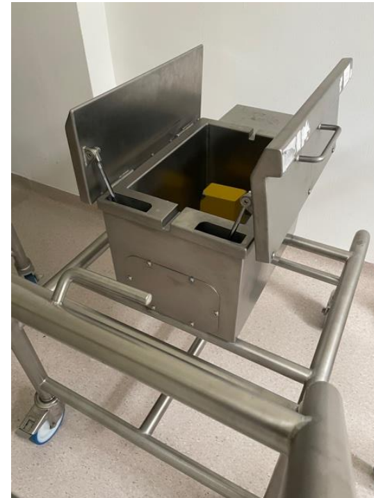
Shielded box on wheels (1 cm perspex, surrounded by 1 cm of lead)
