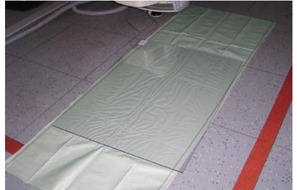
Perspex absorber (1cm) to cover contamination on the floor
