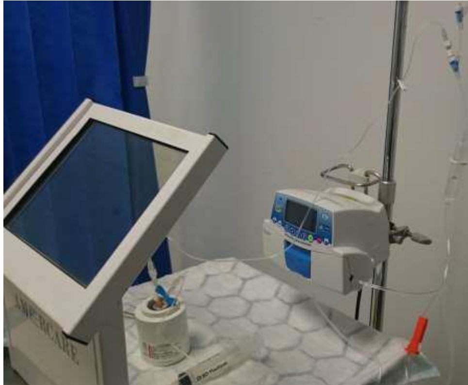
Placement of the shielded via behind a shield of lead glass
