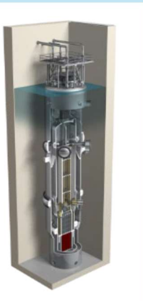
2. NuScale Module including containment and reactor vessel
