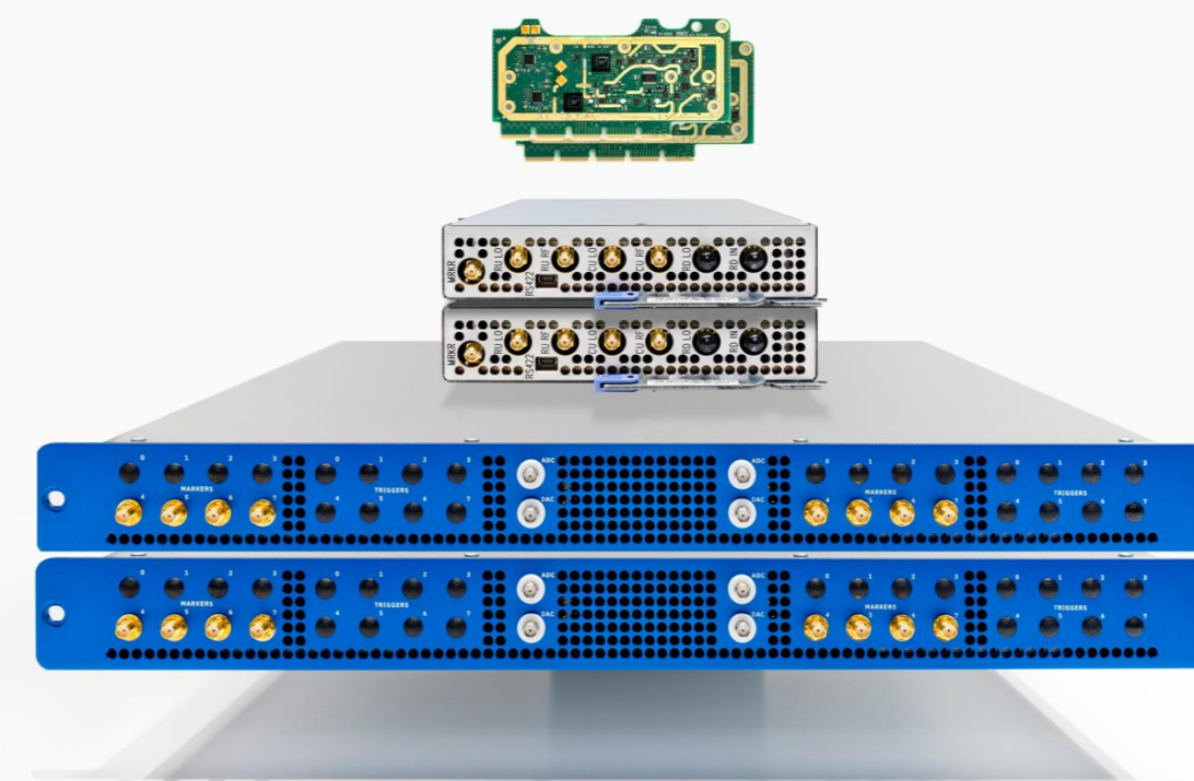
Full-featured 4K cryo-CMOS qubit controller
