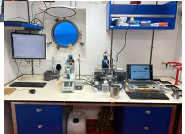
Winkler titration workbench using iodate standards for bottle oxygen measurements
