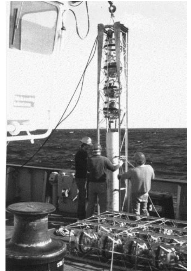
Deep SOFAR float using glass spheres. (photograph, John Gould).
