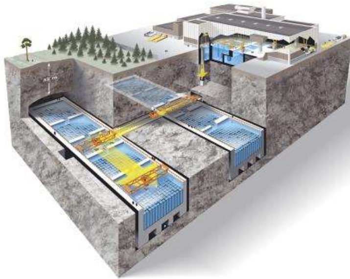
Centralized Wet Storage (Oskarshamn) 8000 tHM
