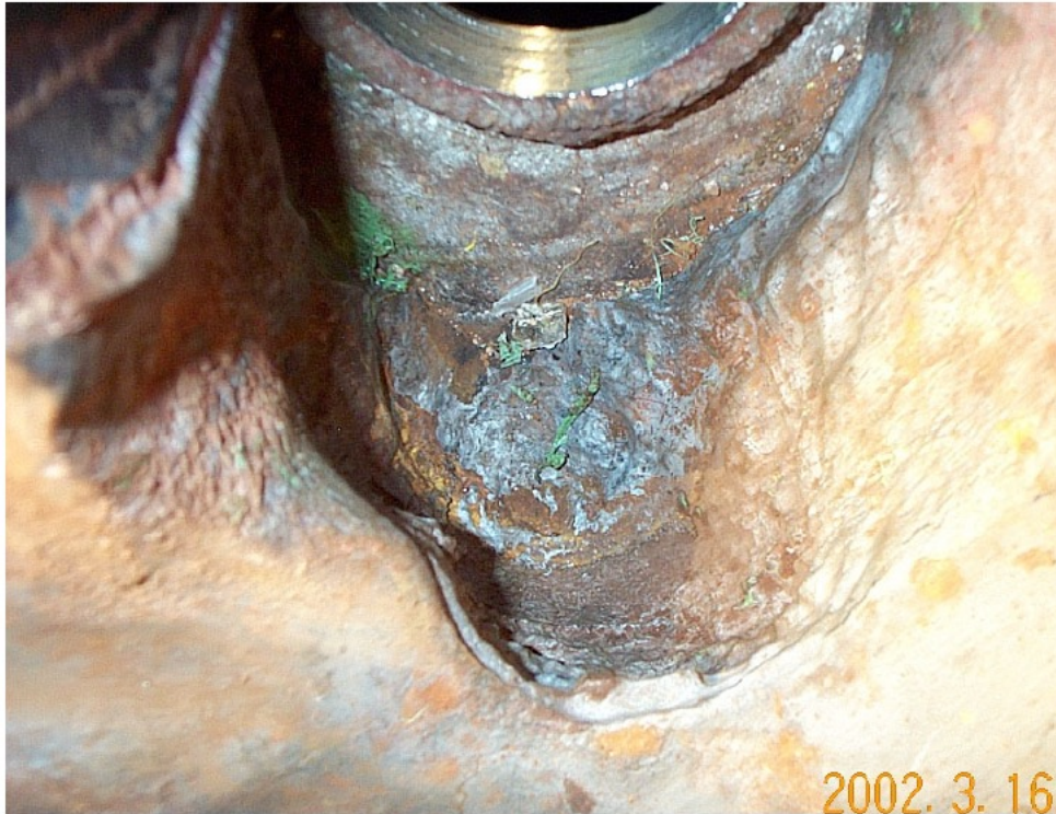
Davis Besse Reactor Vessel Head Degradation Head Cutaway View
