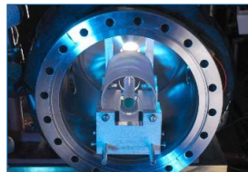
NPL cut-out cavity with 4-point support Webster et al. PRA 75, 011801 (R) (2007)
