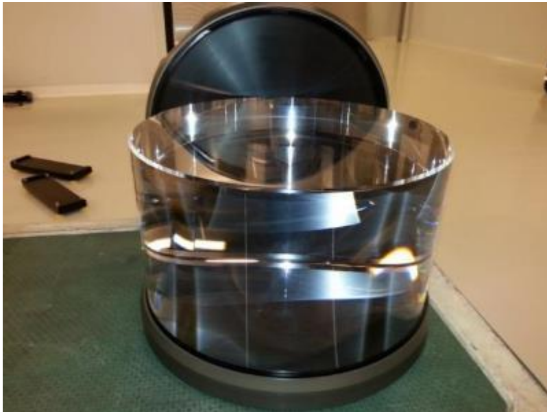
Example of a 3 km arm cavity input mirror (350 mm in diameter, 200 mm thick)
