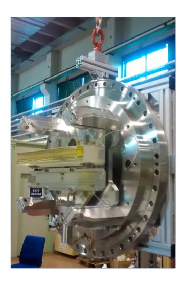
An ellipsoidal mirror focus the FEL on spots of 5 um diameter
