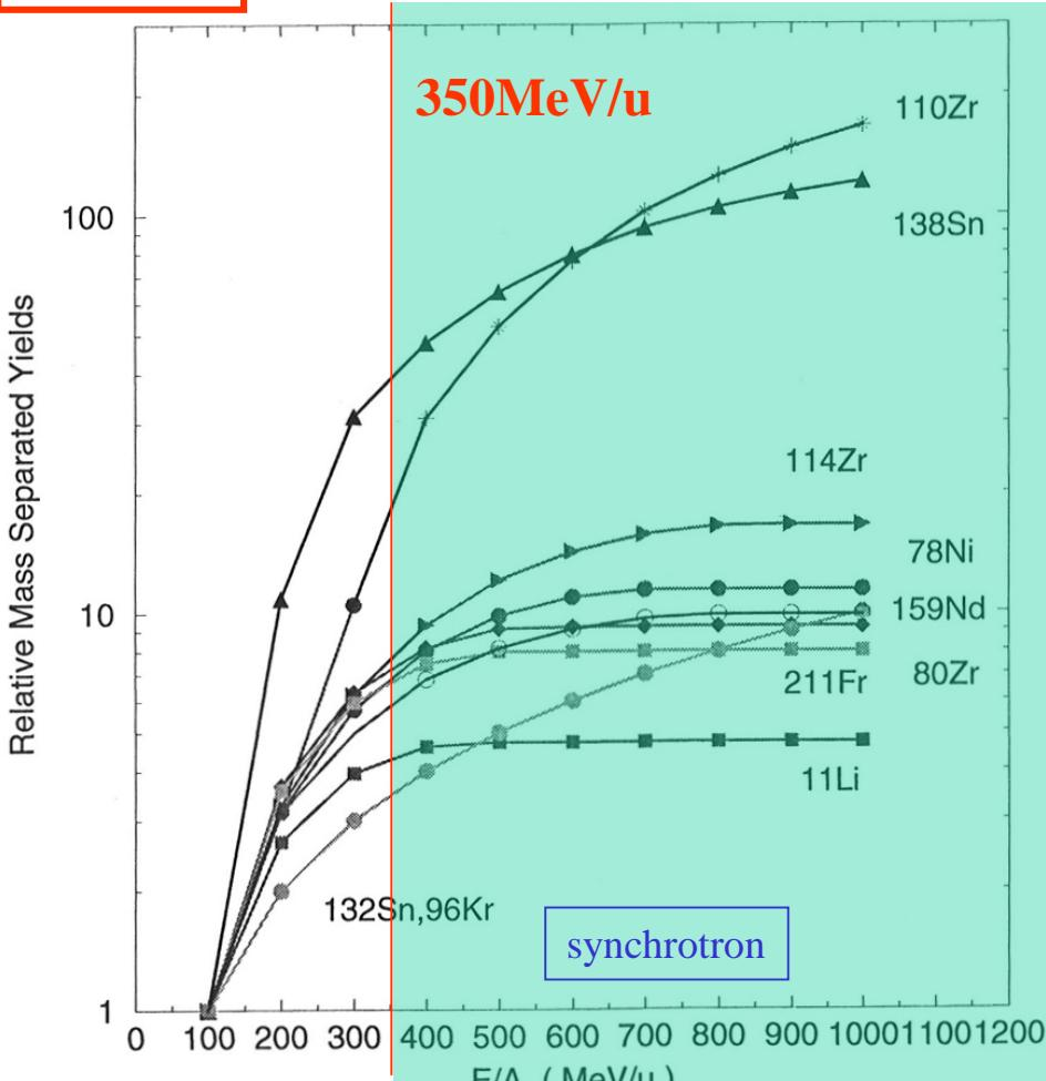
Cyclotron provides more intense beams than synchrotron.
