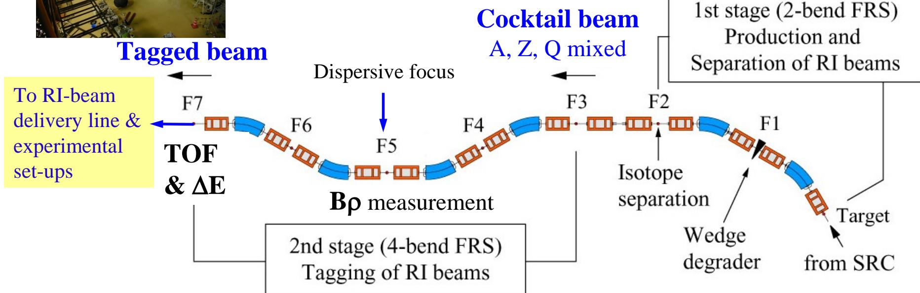
**Identify RI-beam species Z, A/Q by measuring  $\Delta E$ , B $\beta$ , TOF in an event-by-event mode using beam-line detectors on the 2nd stage.** Aim at tagging rate up to  $1 \times 10^6$  pps.
