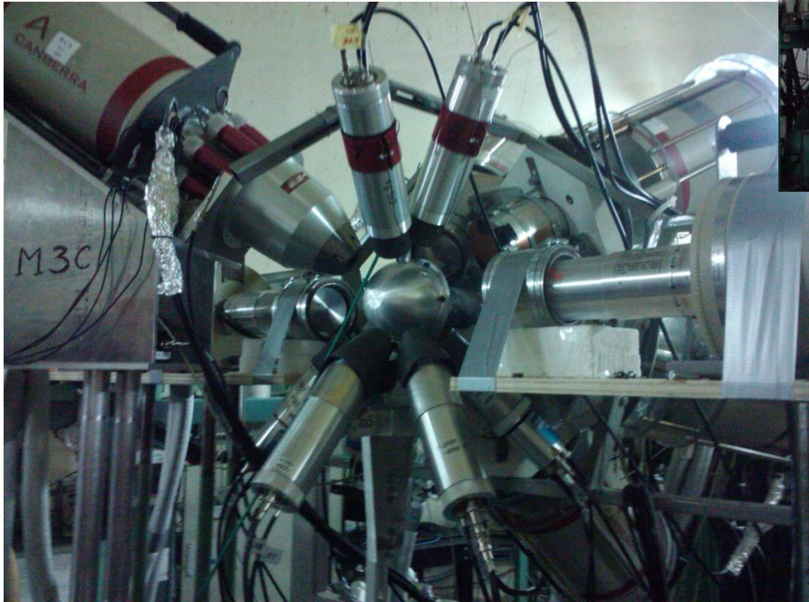
Array 8 HPGe (unsuppressed) and 7 LaBr<sub>3</sub>:Ce detectors
