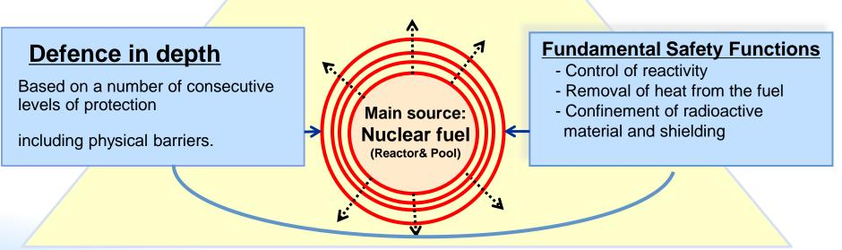
The current implementation of DiD at nuclear power plants comprises **5 levels** of protection and it is based on 4 physical barriers (fuel matrix, fuel cladding, reactor coolant boundary and containment building)
