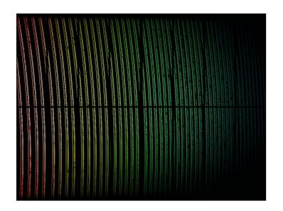
To better understand what I am talking about, I show you what an ESPRESSO spectrum looks like. In this picture you can easily see the cross-dispersed echelle orders, each one split into two fiber traces, dedicated respectively the spectrum calibration source (or the sky) and the target. Simultaneous calibration adds up to the instrument thermo-mechanical stability as a way to maintain a steady calibration for long periods of time.
