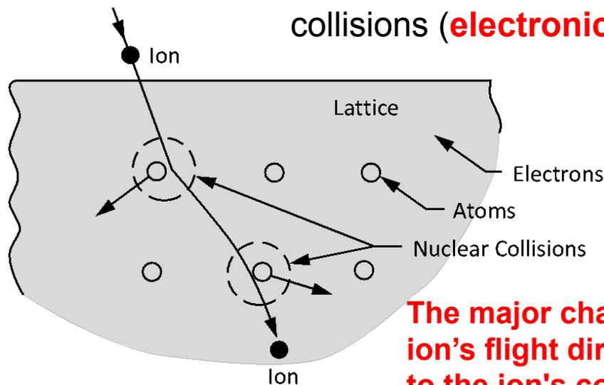
**The major changes in the ion's flight direction are due to the ion's collision with individual lattice atoms (nuclear collisions).**
