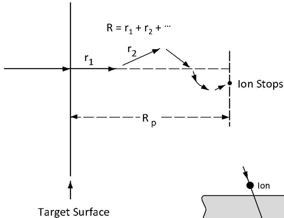
The passage of an energetic ion in a solid during an ion implantation. As the ion travels across the solid, it undergoes collisions with stationary target atoms, which deflect the ion from its initial direction (**nuclear stopping**).
