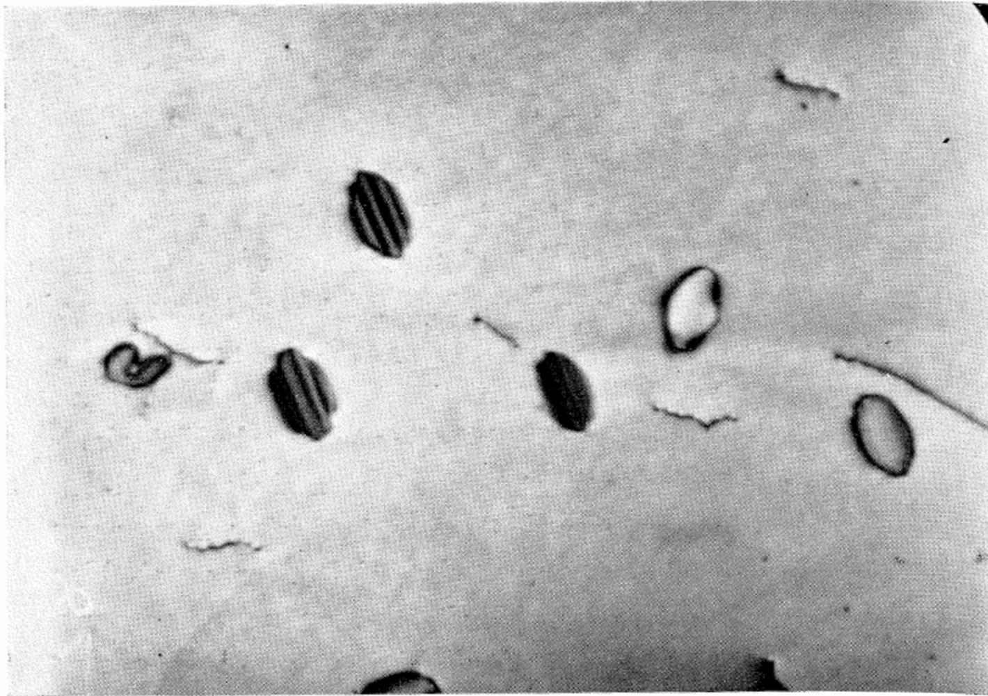
Quenched Al: Hexagonal loops with enclosed stacking fault
