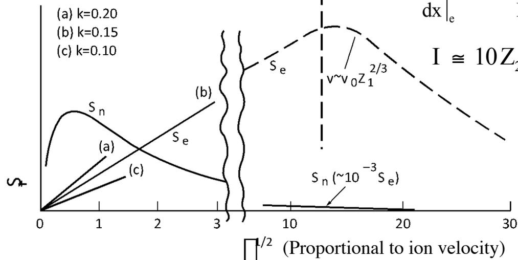
Nuclear energy deposition dominates as the ion slows down, which leads to defect production and damage of the local atomic structure
