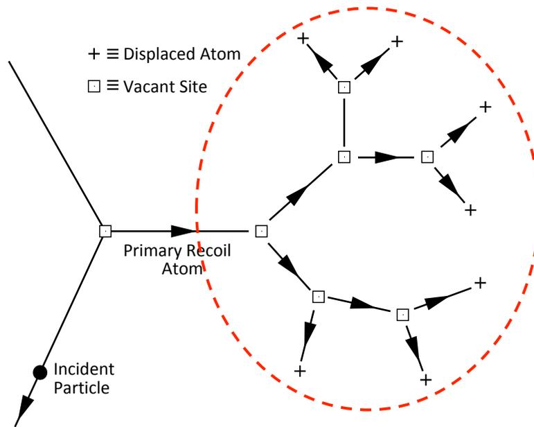
Collisions between ions and target atoms result in the slowing down of the ion. In these collisions, sufficient energy may be transferred from the ion to displace an atom from its original site
