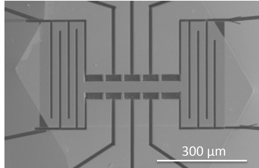
Focused ion beams can be used to sculpt out arbitrary geometries; beyond a 10-20 nm damage layer this process is clean.
