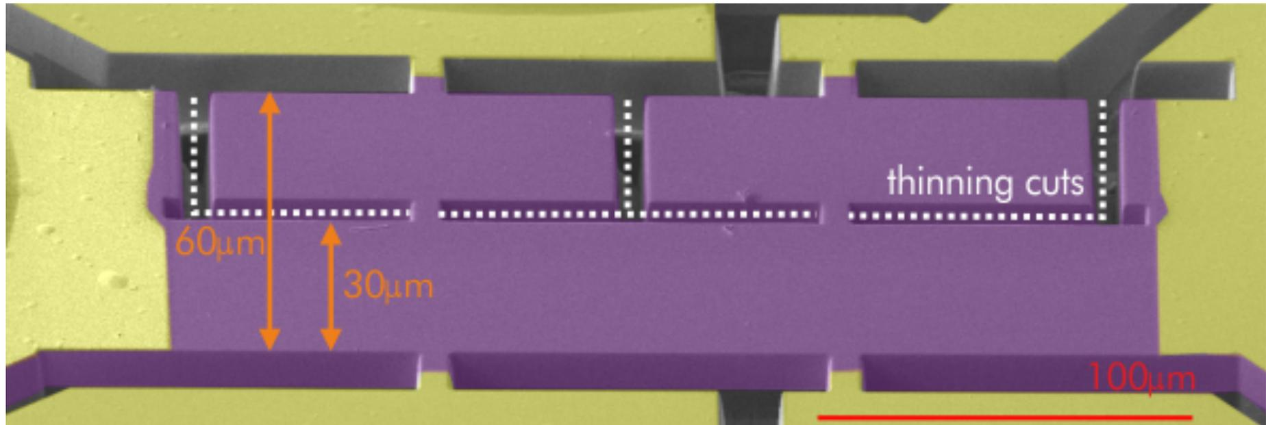
**Experiment:** Successively narrow the channel in factors of 2, measuring the resistance after every step.
