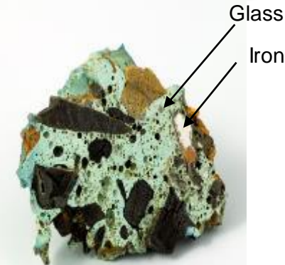
Steel production: Blast furnace slags from iron ore reduction (400 y. in an iron (anoxic burial medium) and clayey environment)
