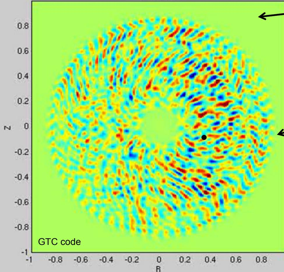
Simulated tokamak turbulent electrostatic potential structure ( $\delta\phi$ )
