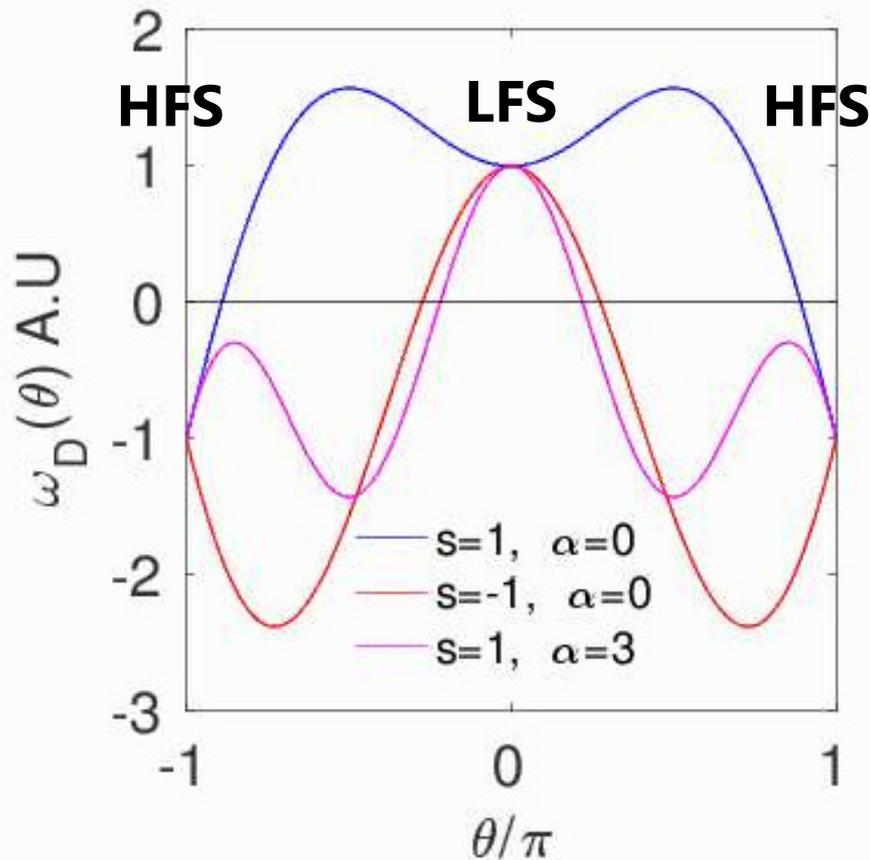
At negative magnetic shear, and for high Shafranov shift, a significant portion of the drift frequency can flip direction, which is highly stabilizing
