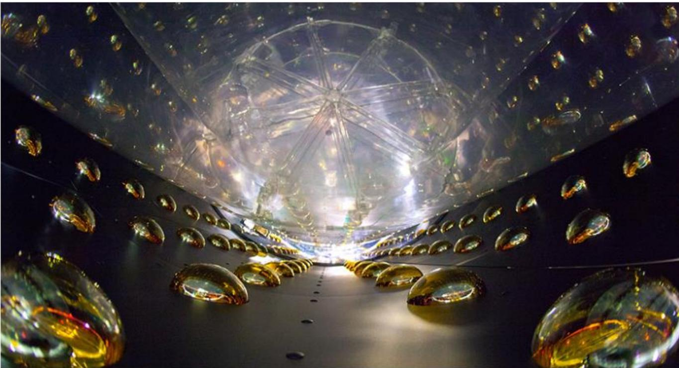
**GHOST FINDER** New results of experiments at the Daya Bay neutrino detector (walls lined with photomultiplier tubes, shown) hint at the existence of a lightweight sterile neutrino, about one-millionth the mass of an electron.
