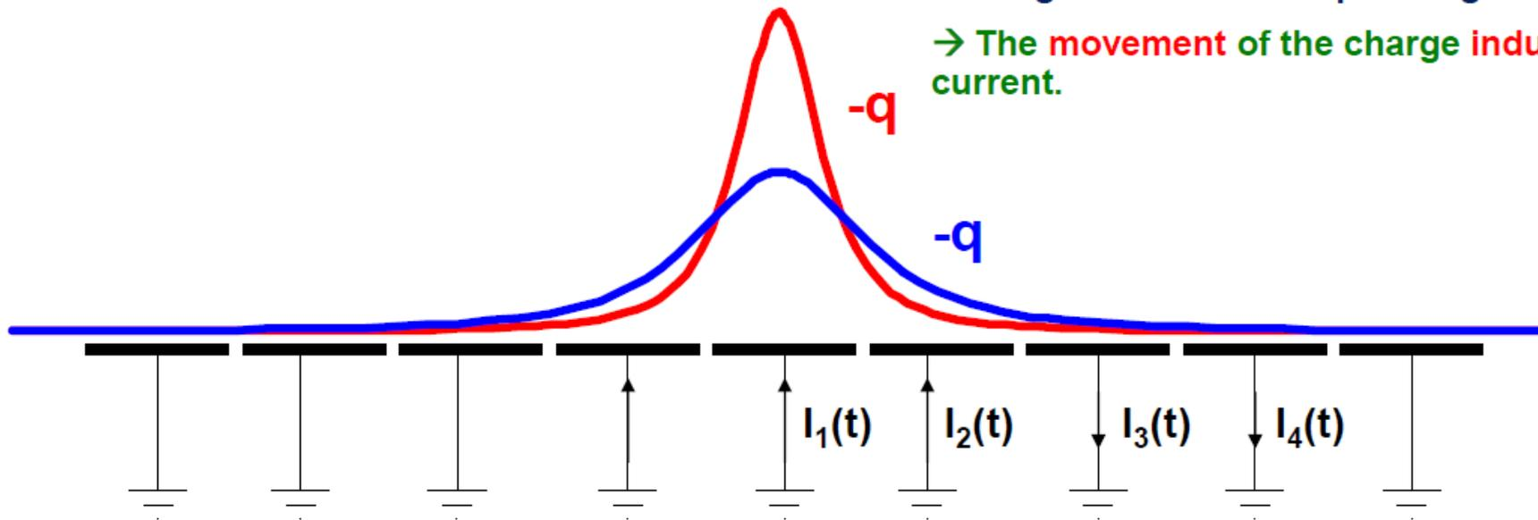
$$Q_1(z_0) = \int_{-\infty}^{\infty} \int_{-w/2}^{w/2} \sigma(x, y) dx dy = -\frac{2q}{\pi} \arctan\left(\frac{w}{2z_0}\right) \quad z_0(t) = z_0 - vt$$
