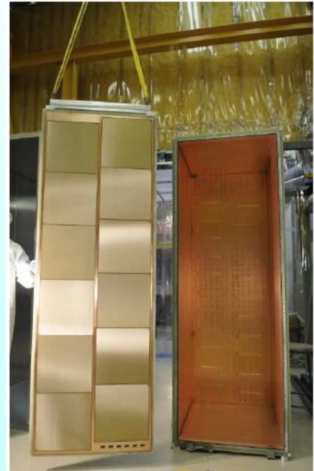
Bulk Micromegas ILC DHCAL first m<sup>2</sup>
