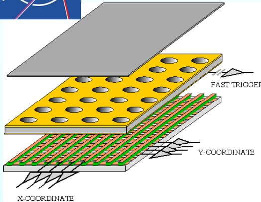
Full decoupling of the charge amplification structure from the charge collection and readout structure.
