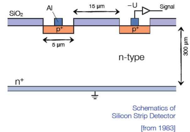
High resistive n-type silicon onto which  $p^+$  diode strips with aluminum contacts are implanted
