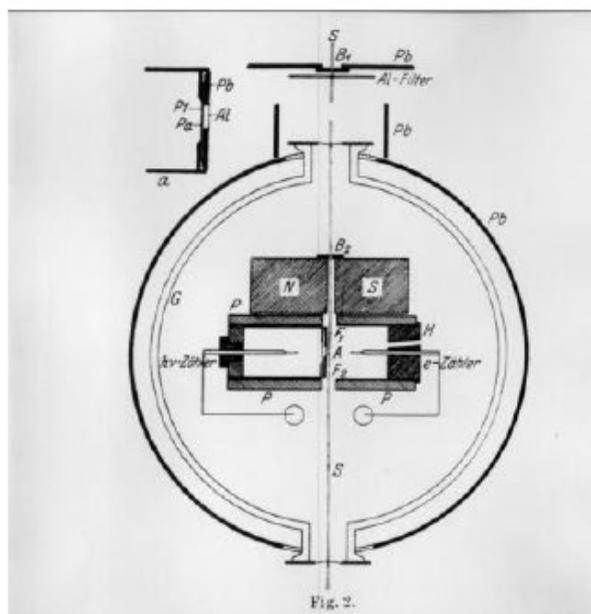
The needle is connected to an electroscope that can detect the produced charge.
