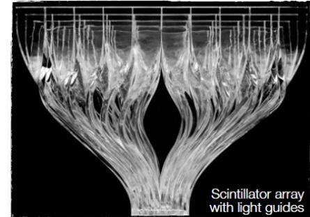
Scintillator array with light guides
