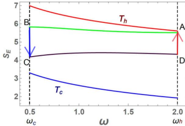
$$\text{Adiabatic efficiency } \eta = 1 - \frac{\omega_c}{\omega_h} \leq 1 - \frac{T_c}{T_h}$$
