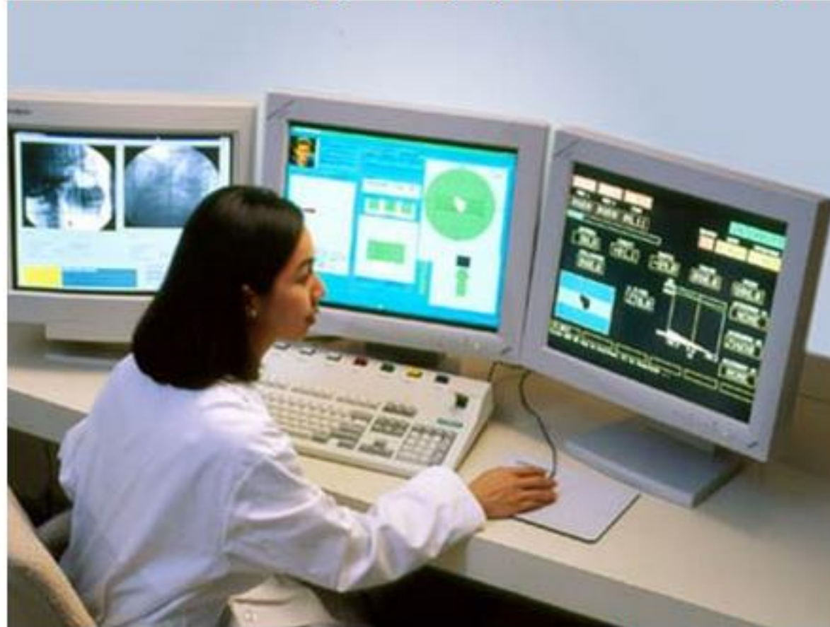
A linear accelerator control console showing all of the functions monitored during a treatment.
