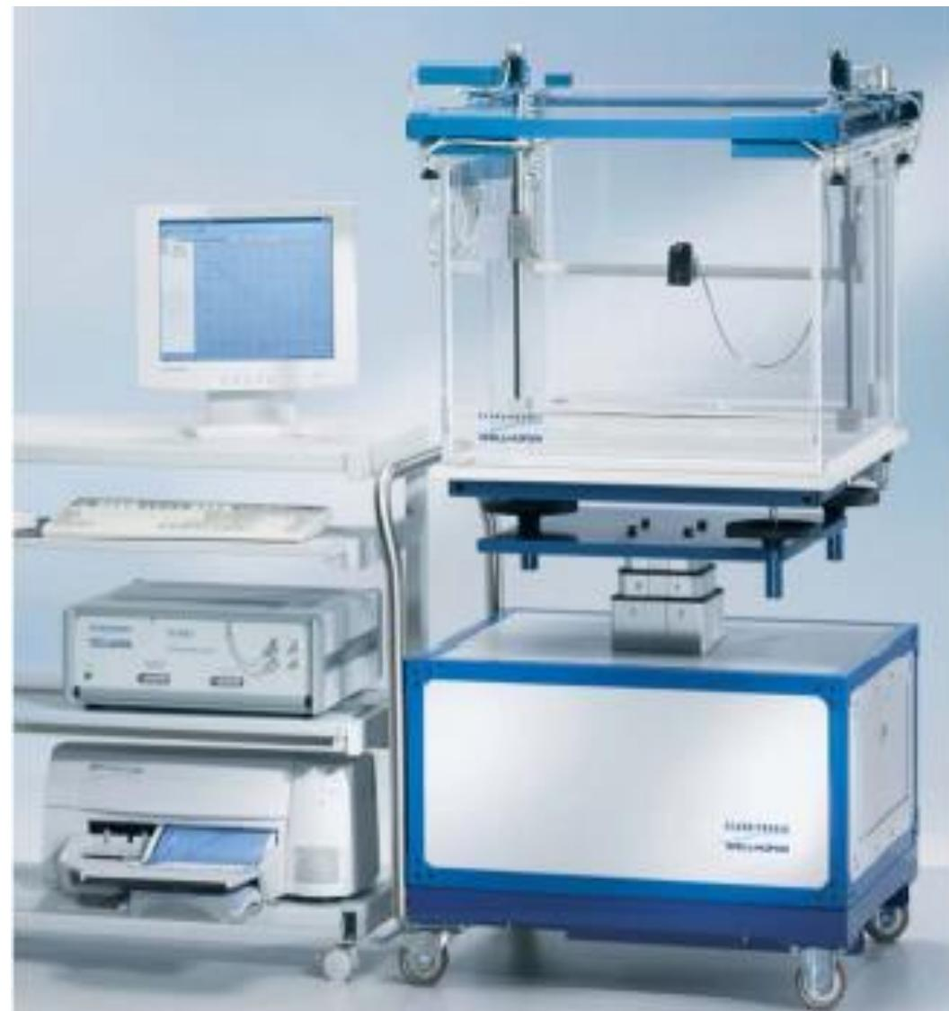
To perform isodose measurement in water with different type of ionization chamber, diodes.
