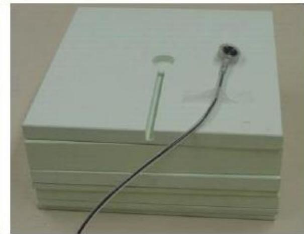
Water equivalent phantom with (a) Farmer-type ion chamber and
