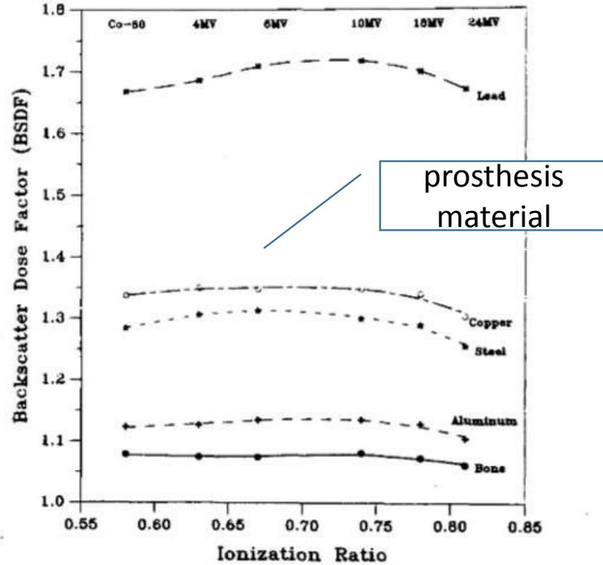
FIG. 5. Backscatter dose factor (BSDF) vs energy of the photon beams plotted as the ionization ratio defined in AAPM Protocol TG-21, for various media.
