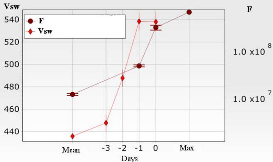
The solar winds speed grows as early as 3 days before the start of the electron flux increase. On Day (-1), it reaches a maximum that lasts 2 days, including Day (0). This growth is characteristic of high-speed streams from large coronal holes.
