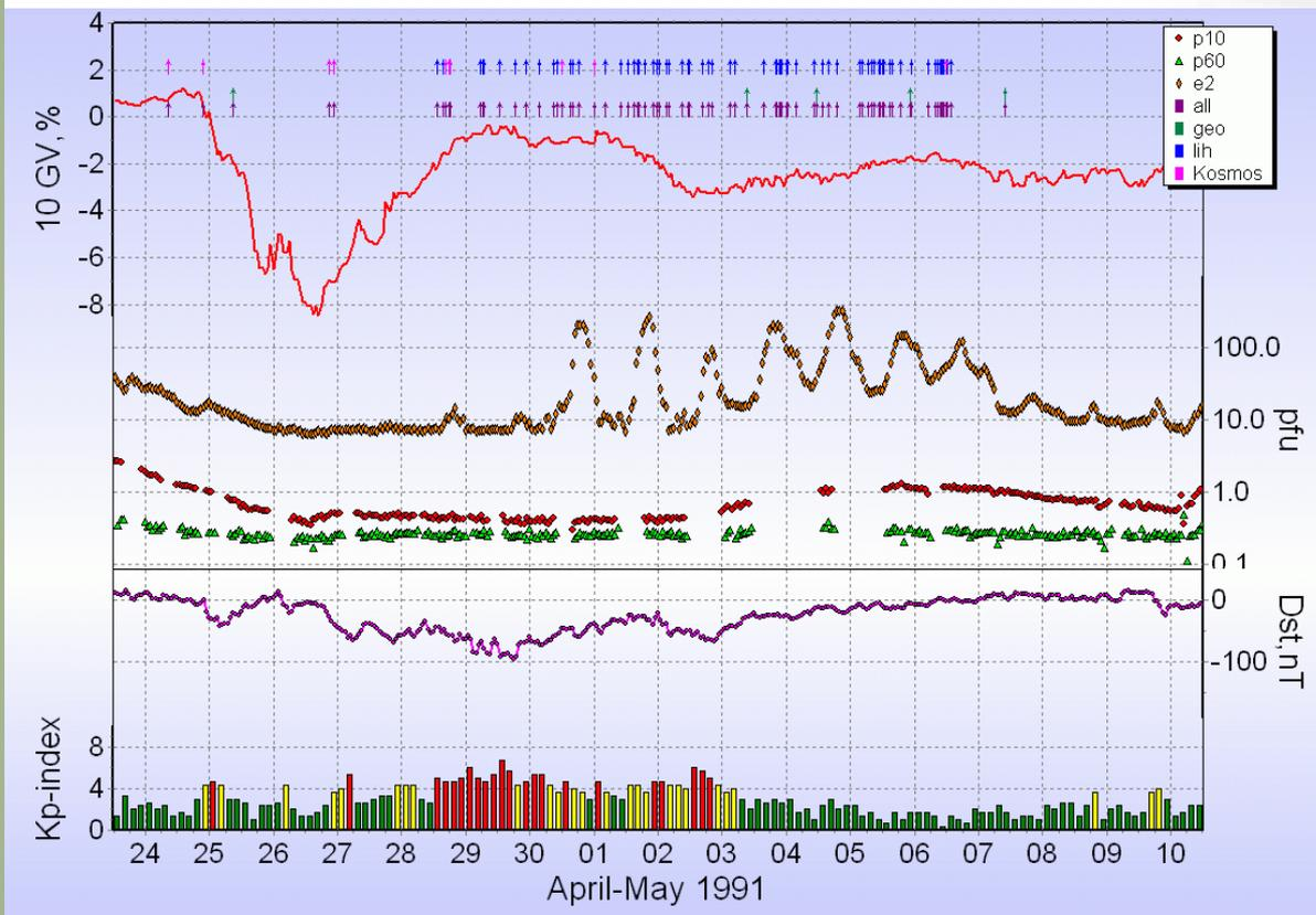
Here the majority of the satellite malfunctions coincides with period of magnetic storm and enhancement of high-energy electron flux. The malfunctions are absent entirely in the high altitude - high inclination group, which played the main role in preceding example. Only a few malfunctions were in GEO group and huge majority – in “blue” group (low altitude - high inclination). We see entirely other subset of satellites comparing with first example.
