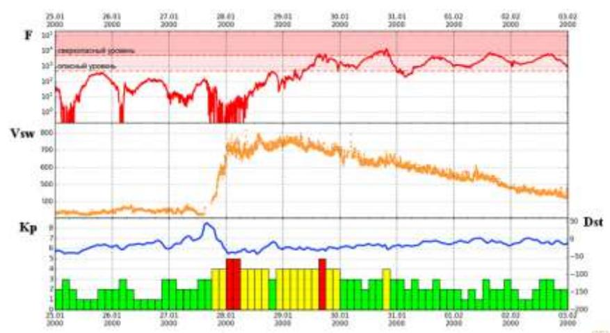
The example of the behavior of the flux of high-energy ( $> 2$  MeV) electrons and other parameters in January - February 2000.
