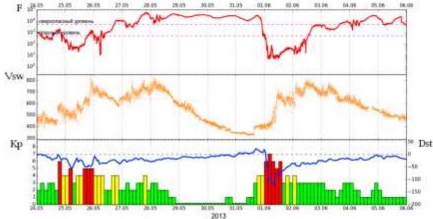
In this work, we assumed that the electron flux begins to grow when the daily fluence exceeds  $10^8$  electrons  $(\text{cm}^2 \text{sr day})^{-1}$ . Increases from this level are typically considered to be dangerous.
