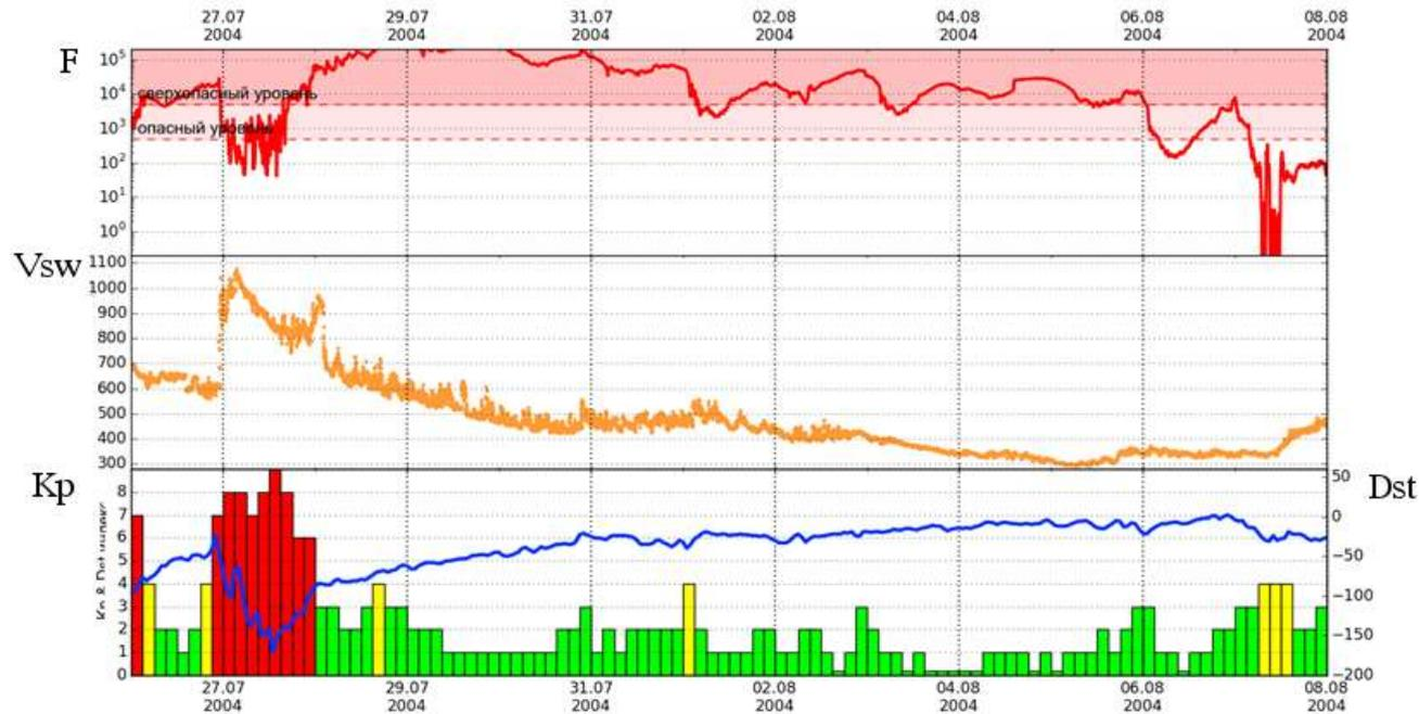
A no less important characteristic of an electron flux increase (in addition to the maximum daily fluence) is probably total fluence  $S$  over the period of growth. In our catalog, the largest total fluence is found for the event lasting from July 28 to August 5, 2004:  $2.6 \times 10^{10}$  electrons  $\text{cm}^{-2} \text{sr}^{-1}$ .
