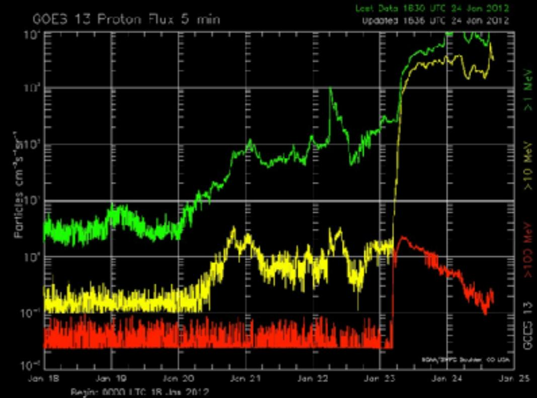
A few times explosions or eruptions will accelerate large amount of particles that travel at almost the speed of light. Such showers of particles consist mostly of protons and it takes less then an hour to reach Earth.
