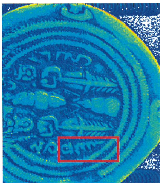
Fig. 12. Analyzed area of the surface of coin inv. no. GR 42791 using CMXRF.
