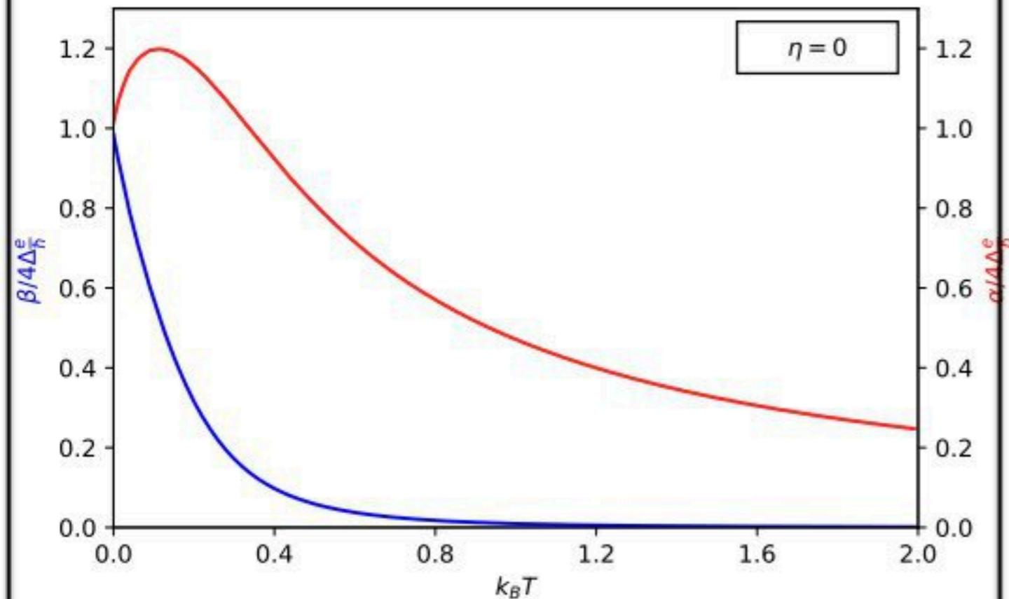
$$\begin{cases} J_c \simeq \frac{4e\Delta_0}{\hbar} (1 + |\Gamma(\theta_V, \theta_\Phi)|) \text{ for } k_B T \ll \Delta_0 \\ J_c \simeq \frac{4e\Delta_0}{\hbar} \frac{\Delta_0}{2k_B T} |\Gamma(\theta_V, \theta_\Phi)| \text{ for } k_B T \gg \Delta_0 \end{cases}$$
