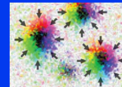
skyrmions or skyrmionic bubbles (with unique rotational sense of the wall) (induced by magnetic fields)
