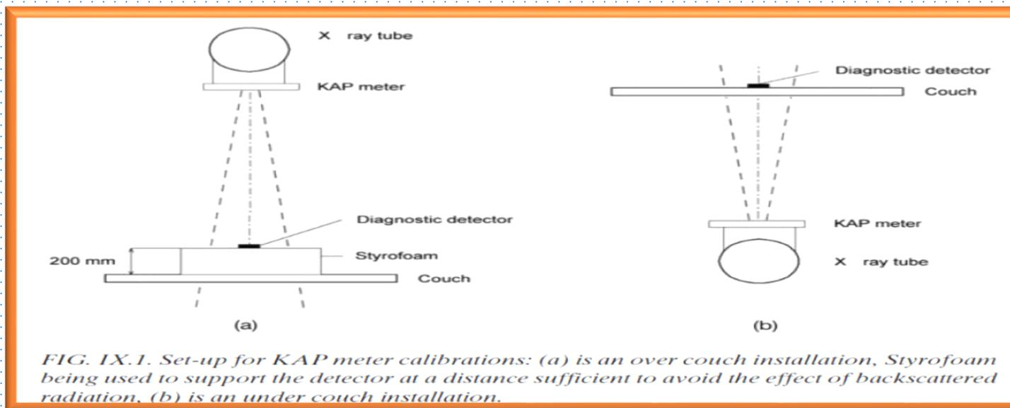
FIG. IX.1. Set-up for KAP meter calibrations: (a) is an over couch installation, Styrofoam being used to support the detector at a distance sufficient to avoid the effect of backscattered radiation, (b) is an under couch installation.
