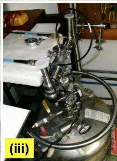
Experimental apparatus for testing superconducting reentrant cavities within a liquid helium cooled dewar.
