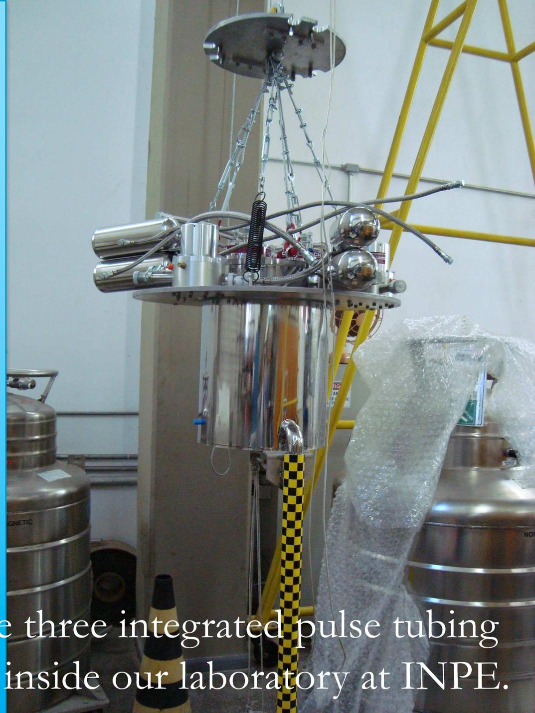
We are going to use these three integrated pulse tubing to cool the sphere down inside our laboratory at INPE.
