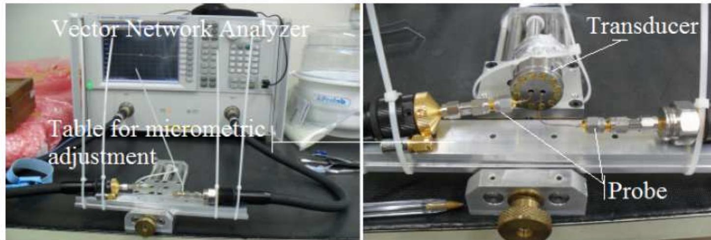
Figure 4. Frequency measurements in the vector network analyzer. The measurements were accomplished by transmission by inserting two probes into the cavity. A table for micrometric adjustment was also used in order to improve the accuracy in the probe position.
