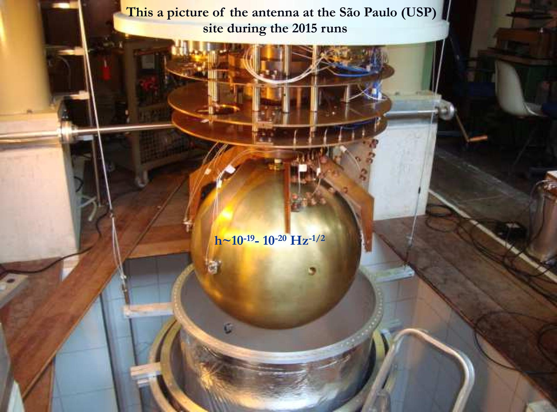
Sphere radius = 0.325 m;  $df/dx = 7.26 \times 10^{14} \text{ Hz/m}^*$
