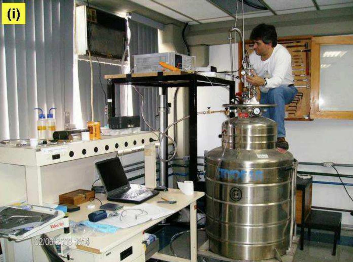
Electrical quality factors ( $Q_e$ ) of several superconducting reentrant cavities at 4.2 K were measured using a liquid helium cooled dewar.  $Q_e$  as high as 300 k were found.
