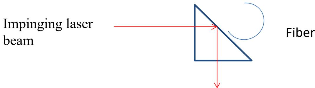
This is the basic set up for coupling between optics elements, such as fiber-fiber or fiber-prism, in measuring devices based on fibers.
