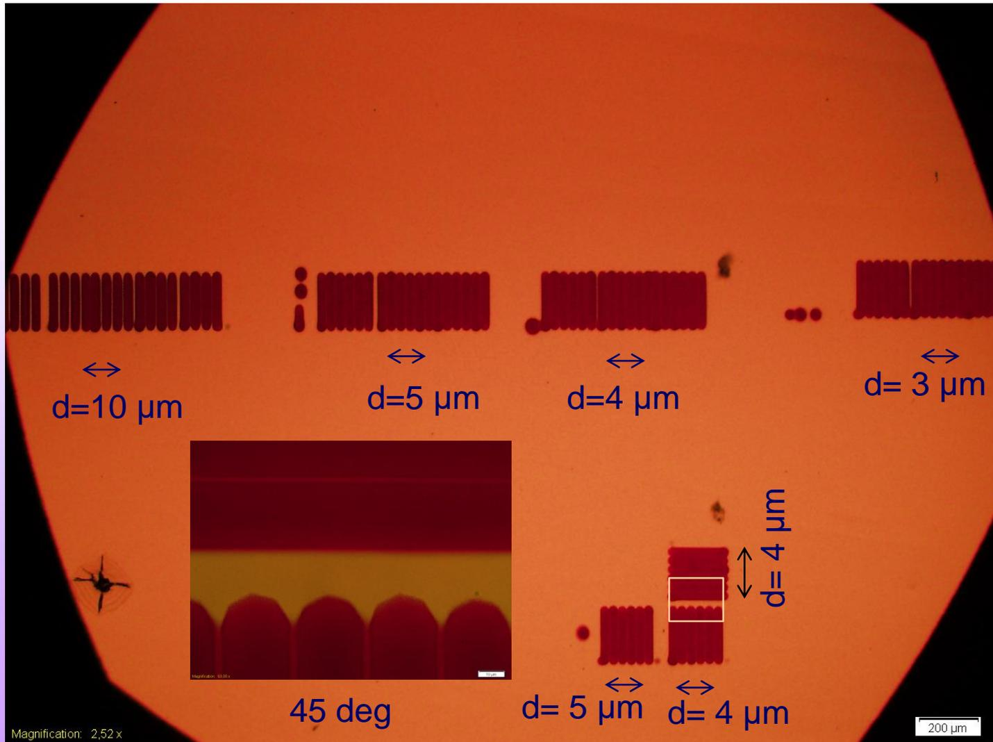
The polarization angle has no spectacular effect among the in contact lower size Au nanoparticles embedded in written patterns except a slight narrowing of the period of the gratings in the horizontal configuration
