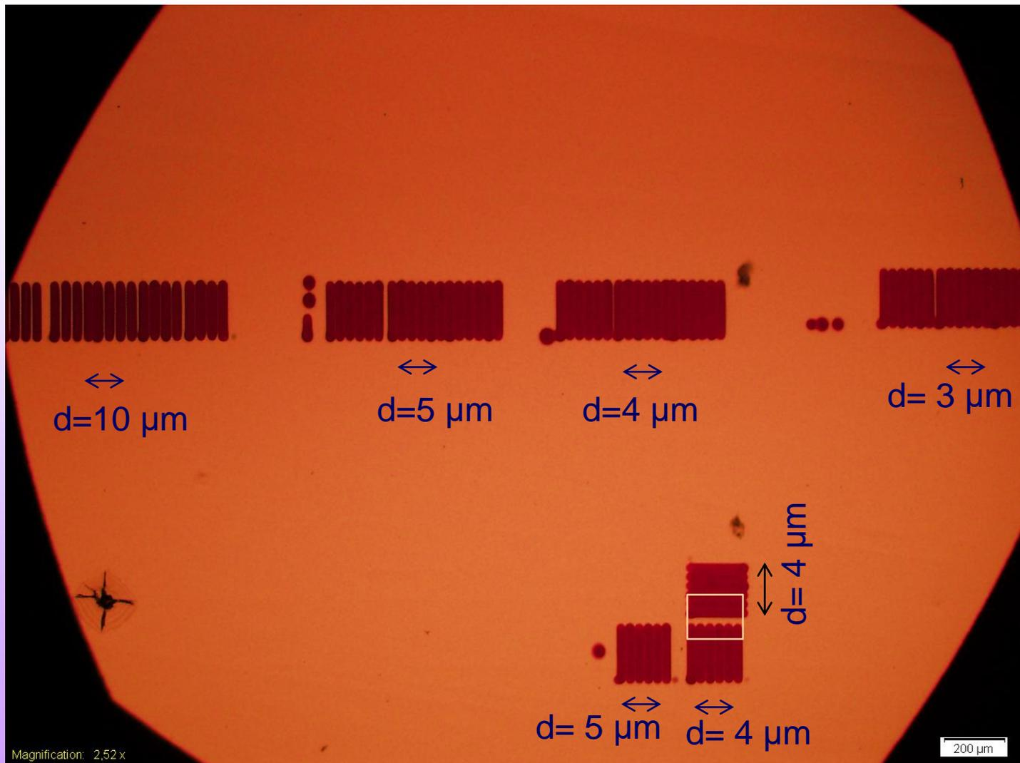
Period of the gratings:  $d = 5 \mu\text{m}$  (V),  $d = 4 \mu\text{m}$  (V and H)
