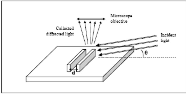
Schematic view of the dark-field arrangement for a metallic double-wire shape
