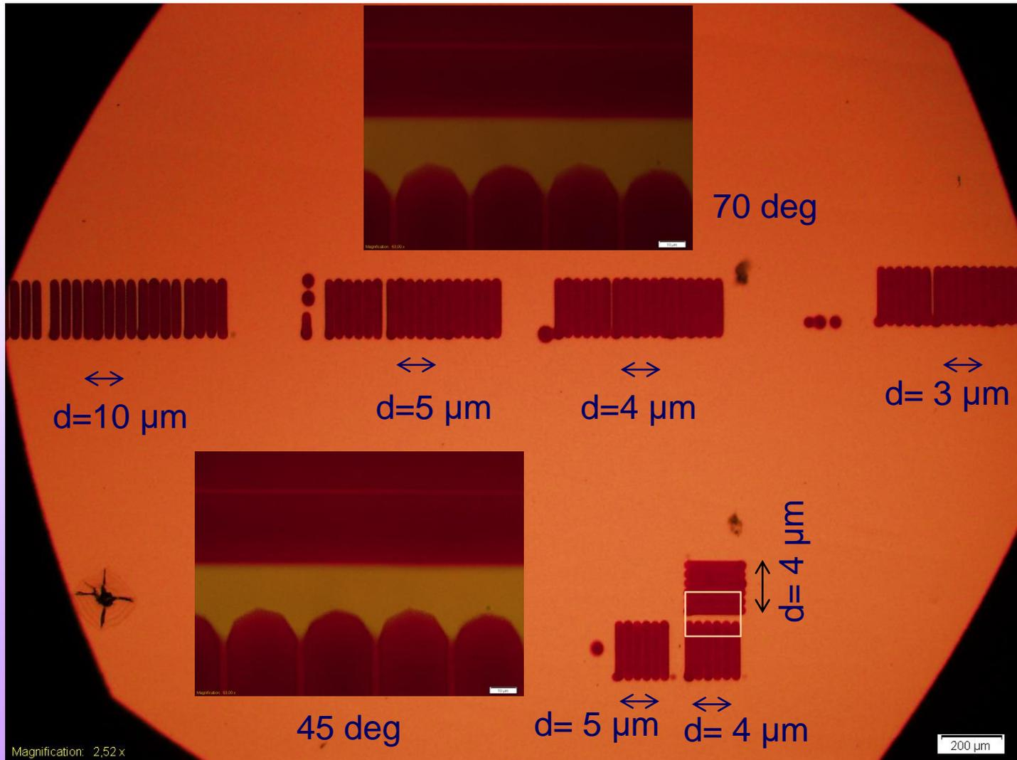
The polarization angle has no effect among in contact lower size Au nanoparticles embedded in the written patterns except attenuating the SPR response due to the light attenuation
