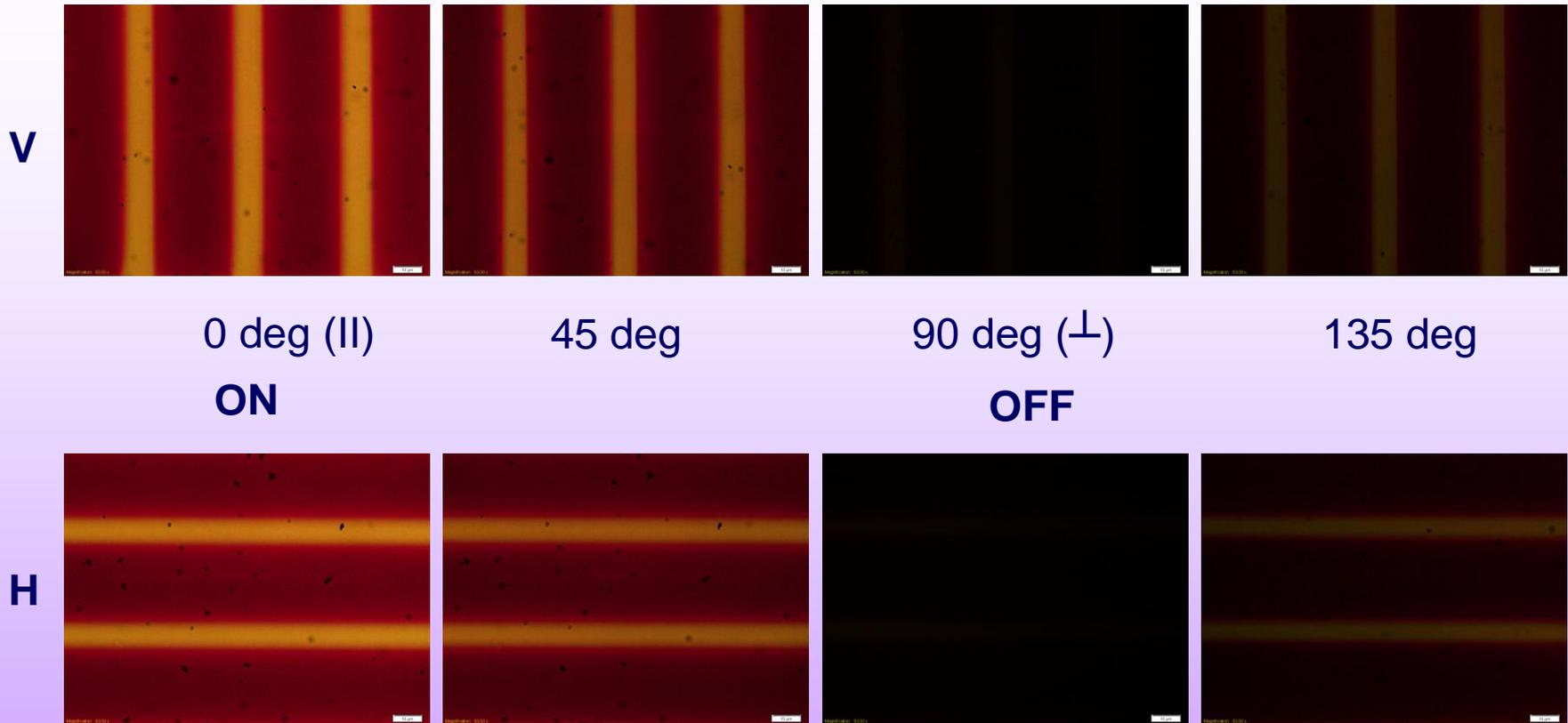
The polarization angle affect the absorbance/transmission of the in contact lower size Au nanoparticles embedded in the written patterns
