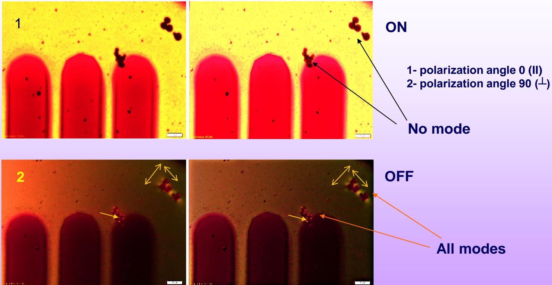
Polarization angle has no effect among ordered and in contact lower size Au nanoparticles embedded in the written patterns
