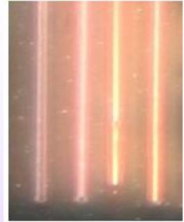
Optical image obtained with metallic double – wire shapes with increasing distances between the walls, from the left to the right
