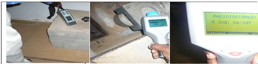
Fig. 1: Detection of Cs-137 orphan radioactive source covered by concrete in the Department of Physics of the University of Yaounde 1; Its identification processing after concrete removal and the screen display of the radiation monitor after identification.
