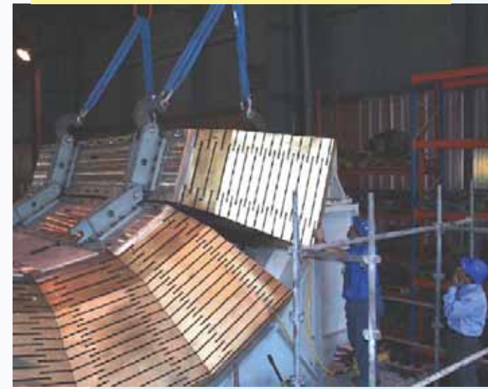
CMS Hadronic Calorimeter: brass and plastic scintillators
