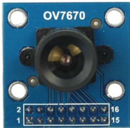
0.3M Pixels CMOS OV7670 CAMERA MODULE
