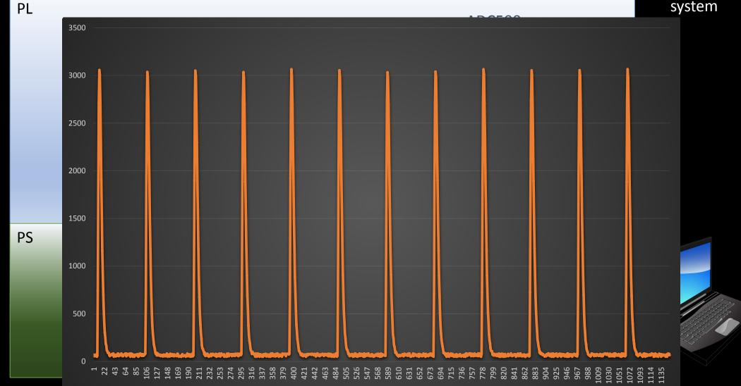
Pulse train was generated on the computer to simulate a photon discharge system
