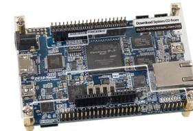
Terasic DE10-Nano (Cyclone V FPGA SoC)
