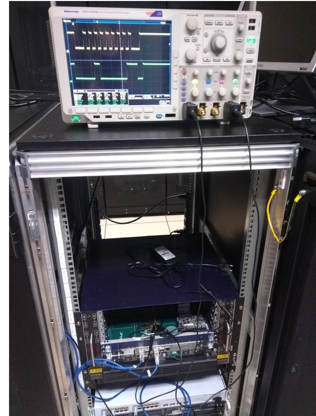
Monitoring IPMB-A with Tek o'scope
