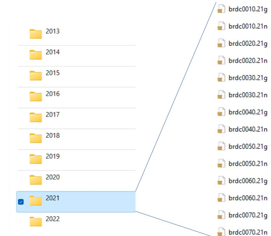
Gg calibration software is a windows package capable of evaluating single-station calibrated TEC from daily RINEX (v2.11) observational (ssssdoy0.yyo) and navigational (brdcdoym0.yyn/g) files from GPS and GLONASS satellites.
