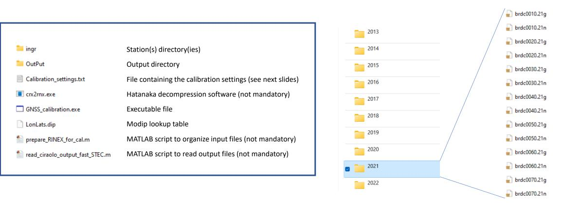
Gg calibration software is a windows package capable of evaluating single-station calibrated TEC from daily RINEX (v2.11) observational (ssssdoy0.yyo) and navigational (brdcdoy0.yyn/g) files from GPS and GLONASS satellites.
