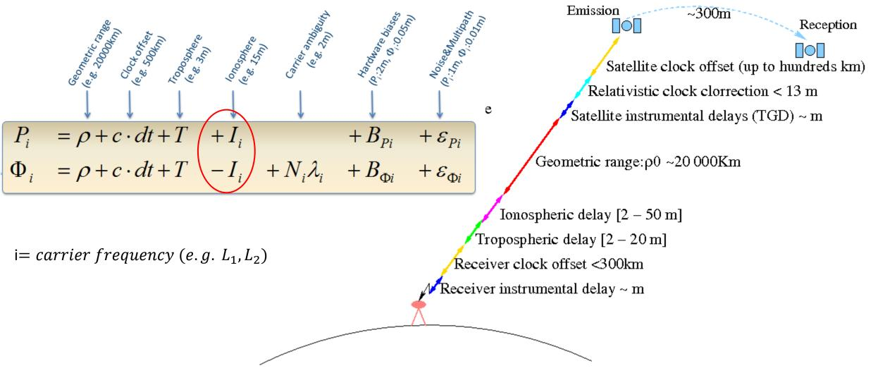
The ionosphere will introduce a delay of the modulation (the code measurement will be larger than in vacuum), and an advance of the carrier phase (the carrier phase measurement will be smaller than in vacuum).
