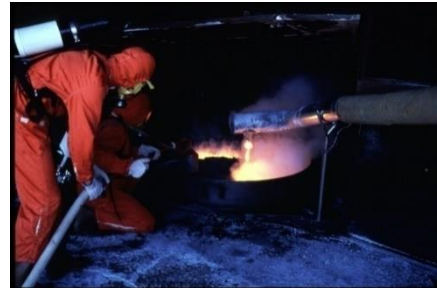
Extinguished with Marcalina powder (sodium carbonate, lithium carbonate and graphite)
