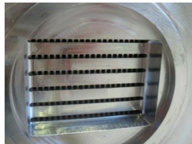
Gas channels entry
