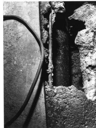
NaH deposits on cold wall (EPINAR experiment)
