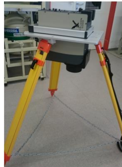
Figure 3 FALCON mounted on tripod, without (left) and with (right) plastic protective cover to shield connectors.
