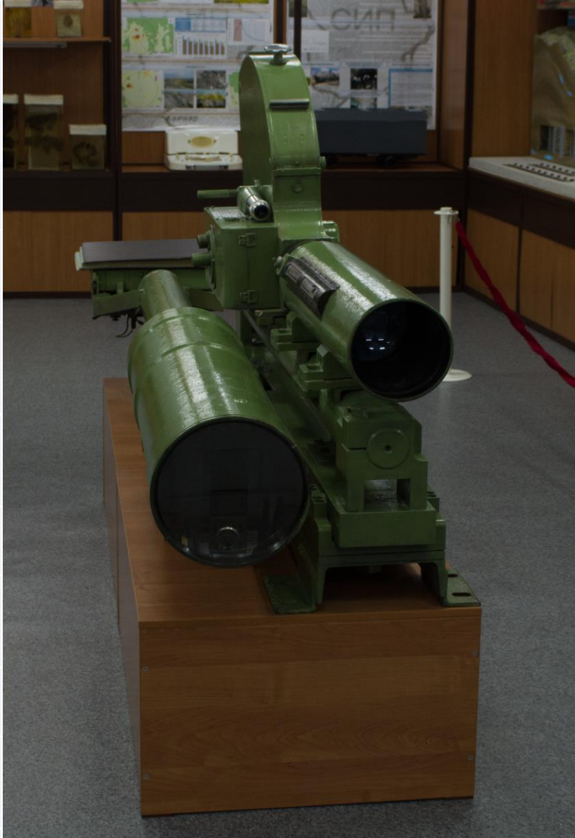
High speed camera: 1 000 000 frame/s
