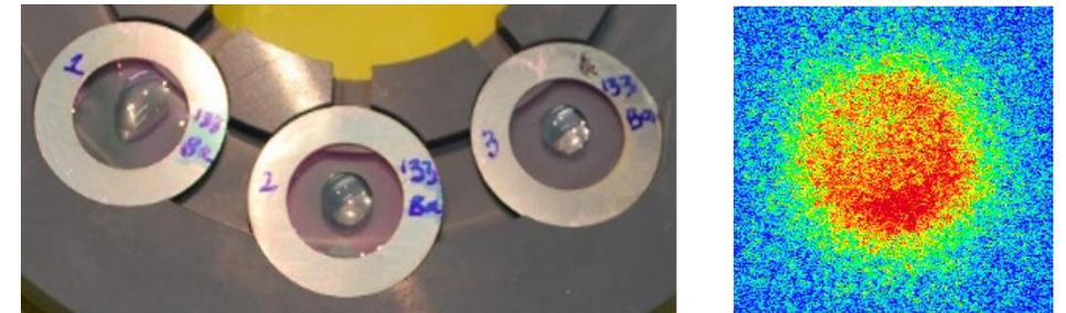
Unsealed sources: 0.5 to  $0.7 \mu\text{m}$  thick
