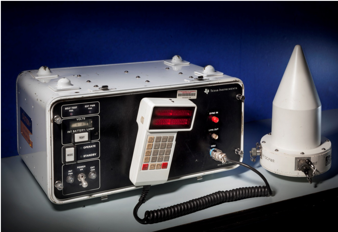
TI 4100 NAVSTAR Navigator Multiplex Receiver designed by Phil Ward for Texas Instruments (1981)
