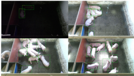
FIGURE 8. Four sample images from our pig detection test set processed by the Faster R-CNN with the feature extraction layers pre-trained on ImageNet, the rest pre-trained on Pascal Visual Object Classes Challenge 2007 and an additional fully-connected layer for the pig dataset. Detections to the left of the red wall are ignored. The top left image is from the low-light test segment. The top right image is from the densely packed test-segment. The bottom left image is from the overexposed test segment. The bottom right image is from the many pigs test segment.
